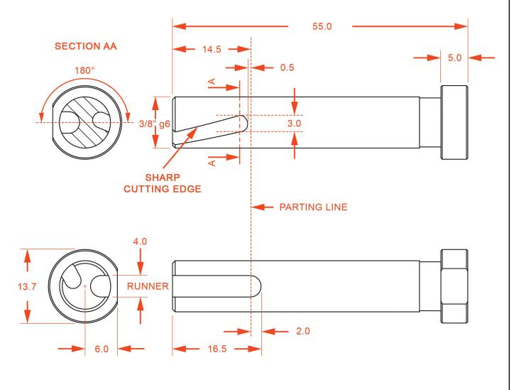
\*Ejector plate must be held back during mould opening time.
